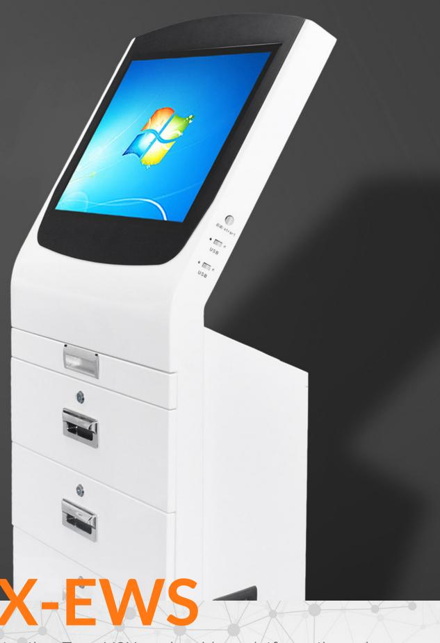
Connected to the TeamVOX main video platform through a dedicated link to a private cloud, the **TVX-EWS** workstations provide the safe keeping and management of video evidence provided by TVXBC1 body cams in the field.
